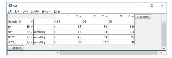
To read the file into **Gtplot**, select **File** → **Open** → **Scatter Data...**. If some of the data points lie outside the plot's axis range, press **Ctrl+Z**. Clear scatter data from a diagram on the **Open** → **Scatter Data...** dialog, with the **OFF** button.
