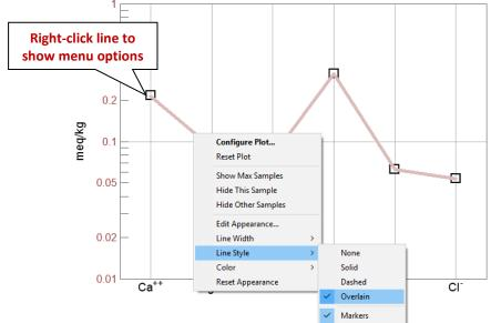
A **left-click** on an aspect causes it to be "selected". An aspect has been selected when its color changes, as in the case of lines, or when it is surrounded by manipulation handles, in the case of text or markers. Change the size of text, markers, and, in the case of the XY Plot, the plot itself by dragging the sizing cursors. Adjust the placement of the plot
