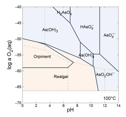
Interior broken lines show mosaic boundaries for sulfur speciation. Subdiagrams in the mosaic, from upper left to lower right, are for the species  $HSO_4^-$ ,  $SO_4^-$ ,  $H_2S(aq)$ ,  $HS^-$ , and  $S^-$ . The basal broken line (black) is the stability limit for water under reducing conditions at 1 atm pressure.
