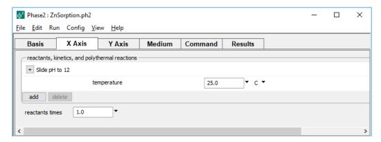
slides pH from its initial value of 4 at the left of the diagram, to 12 at the right.
