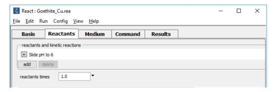
sets a sliding pH path. In the calculation results, copper sorption on goethite increases with pH  $\,$
