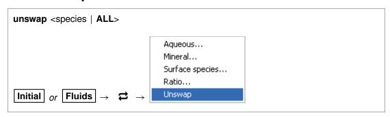
Use the "unswap" command to reverse a basis swap. The swap reversal operates on either the initial system, a boundary fluid, or globally on all fluids, depending on the current input scope (see the "scope" command). Example:
