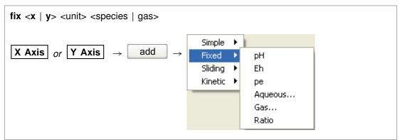
Use the "fix" command to hold the activity of a species, fugacity of a gas, or an activity ratio constant over the course of the staging path ("y") or the scanning paths ("x"). The <unit> can be "activity" or "fugacity" ("a" or "f" for short), "ratio", "pH", "pe", or "Eh", or it can be omitted. Examples:
