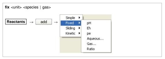
Use the "fix" command to hold the activity of a species, fugacity of a gas, or an activity ratio constant over the course of a run. The <unit> can be "activity" or "fugacity" ("a" or "f" for short), "ratio", "pH", "pe", or "Eh", or it can be omitted. Examples:
