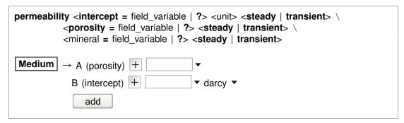
You use the "permeability" command to set the correlation by which the program calculates sediment permeability. **Phase2** calculates this value as a reported variable consistent with **X1t** and **X2t**, but does not use it in its calculations.
