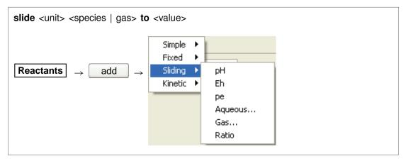
Use the "slide" command to linearly adjust the activity of the specified species, fugacity of the gas, or an activity ratio toward <value>, which is attained at the end of the path. Note that the interpolation is made linearly on the logarithm of activity or fugacity if <value> is set as a log, and that <unit> can be "activity" or "fugacity" ("a" or "f" for short), "ratio", "pH", "pe", or "Eh", or omitted. Examples:
