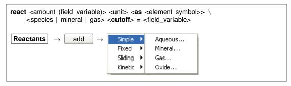
Use the "react" command (abbrev.: "rct") to define the reactants for the current simulation. To set a kinetic rate law for a reactant, use the "kinetic" command.
