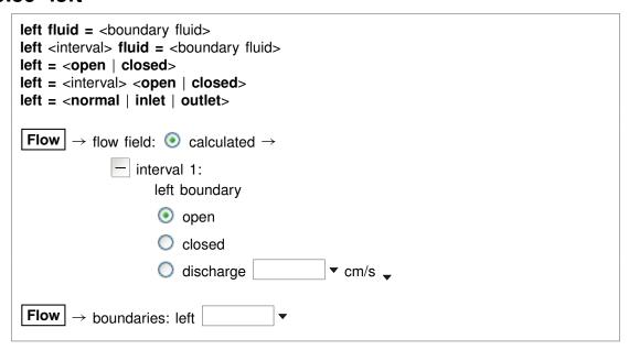
Use the "left" command to control the boundary condition at the left side of the domain: the fluid to appear at the boundary, whether the boundary is open or closed, and whether solutes can diffuse and disperse, and heat conduct, across the boundary.
