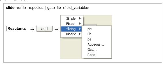
Use the "slide" command to linearly adjust the activity of the specified species, fugacity of the gas, or an activity ratio toward <value>, which is attained at the end of the path. Note that the interpolation is made linearly on the logarithm of activity or fugacity if <value> is set as a log, and that <unit> can be "activity" or "fugacity" ("a" or "f" for short), "ratio", "pH", "pe", or "Eh", or omitted. Examples:
