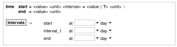
Use the "time" command (abbrev.: "t") to set the time span (keywords "start" and "end") of the simulation, and the start times for individual simulation intervals. The starting time for the run, by default, is zero, and the default end time is 1 day. Unit choices are listed in the **Units Recognized** chapter in the **GWB Reference Manual**; "day" is the default. Examples:
