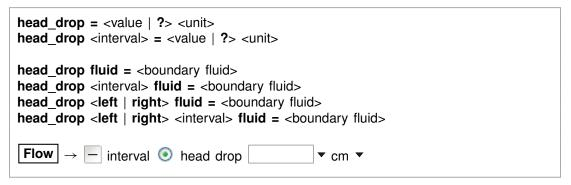
Use the "head\_drop" (also: "pot\_drop") command to set a value for the decrease in hydraulic head (in length units) or hydraulic potential (in units of pressure) across the medium. This decrease provides the driving force for fluid flow. The program sets hydraulic head or potential along the left boundary to the value specified in the command, and sets head or potential along the right boundary to zero.
