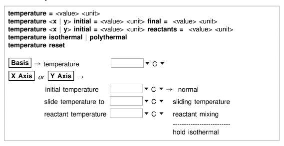
Use the "temperature" command (also: "T") to set the temperature of the system or reactants. The **Units Recognized** chapter in the **GWB Reference Manual** lists possible units, which default to "C". Examples:
