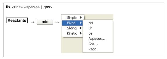
Use the "fix" command to hold the activity of a species, fugacity of a gas, or an activity ratio constant over the course of a run. The <unit> can be "activity" or "fugacity" ("a" or "f" for short), "ratio", "pH", "pe", or "Eh", or it can be omitted. Examples:
