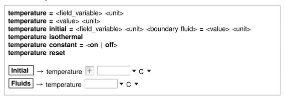
Use the "temperature" command (also: "T") to set the temperature of the initial system or the boundary fluids. The **Units Recognized** chapter in the **GWB Reference Manual** lists possible units, which default to "C". By default, the initial system and boundary fluids are set to 25°C and, in the absence of a heat source, the simulation proceeds isothermally.
