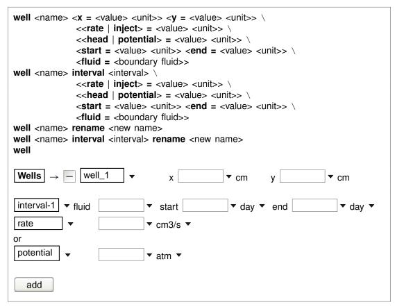
Use the "well" command to define wells and set well properties. Create a well by issuing the "well" command with a new well name. If you omit the well name from the command line, the program assumes the command applies to the most recently referenced well, the name of which is given by typing "well" without arguments. Type "show wells" to see a list of wells and their properties.
