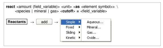
Use the "react" command (abbrev.: "rct") to define the reactants for the current simulation. To set a kinetic rate law for a reactant, use the "kinetic" command.
