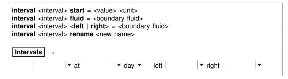
The "interval" command sets the properties of a named simulation interval, creating it if necessary. The first interval is named "start", and the terminating point for the run is labeled "end", but you can create any number of intervening intervals.
