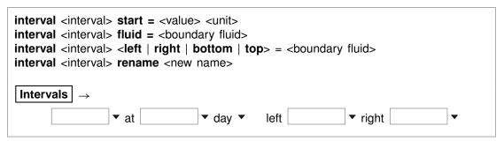
The "interval" command sets the properties of a named simulation interval, creating it if necessary. The first interval is named "start", and the terminating point for the run is labeled "end", but you can create any number of intervening intervals.
